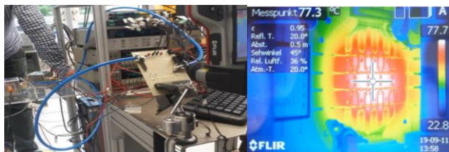
Fig. 5. Measurement setup for the thermal demonstrator boards (left) and Temperature on the surface of the PCB (right).
