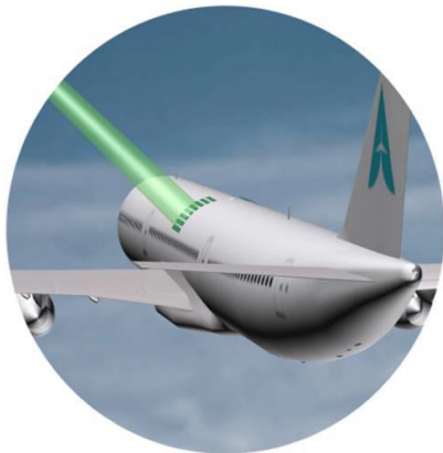
Fig. 1. Conformal and structural integration of Ku-band electronically steerable phased array antenna
