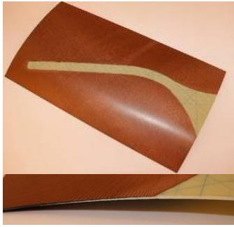
Fig. 4. Preliminary sample of the winglet skin: top view and cross-section of the scarfed GFRP window.
