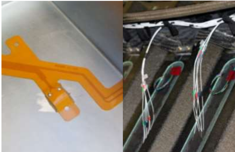
Figure 4: Wiring and piezo transducer integrated in smart layer (left) and piezo transducers with external wiring (right)
