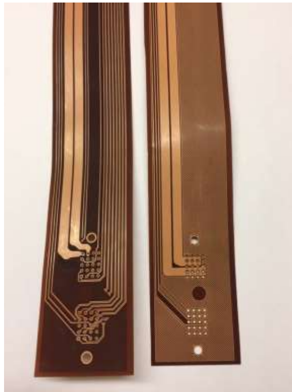
Figure 12: Data and power tracks on a single PCB
