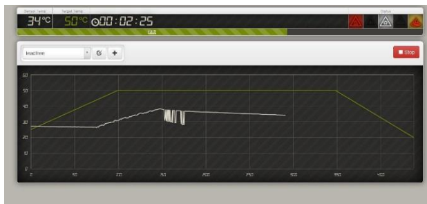
Figure 9: GUI of the control device for heatable moulds during test phase
