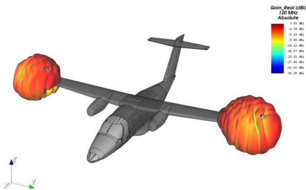
Figure 6: simulated antennas radiation
